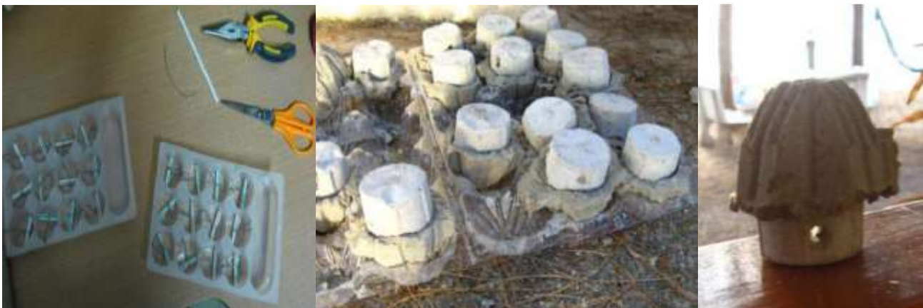
Figure 5: Preparation of settlement "mushrooms" (True, 2009); one mushroom is ca. 6cm high and has a diameter of 2.5 cm to 4 cm
